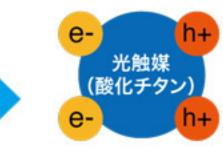
1. Irradiate the photocatalyst 2. Generation of electrons and holes from photocatalyst (titanium oxide)
